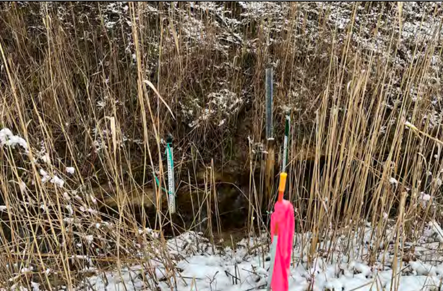
11. Looking at Staff Gauge Location Along Northeast Corner. Ditch Open but Flow not Observed. Some slope drainage into ditch.
