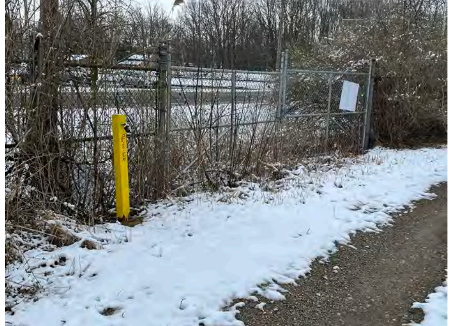
14. Another Perimeter Fence Gate Locked and Signage Postage. Gates Only Used for Maintenance Access if Necessary. Piezometer 96-W-12R, Locked.
