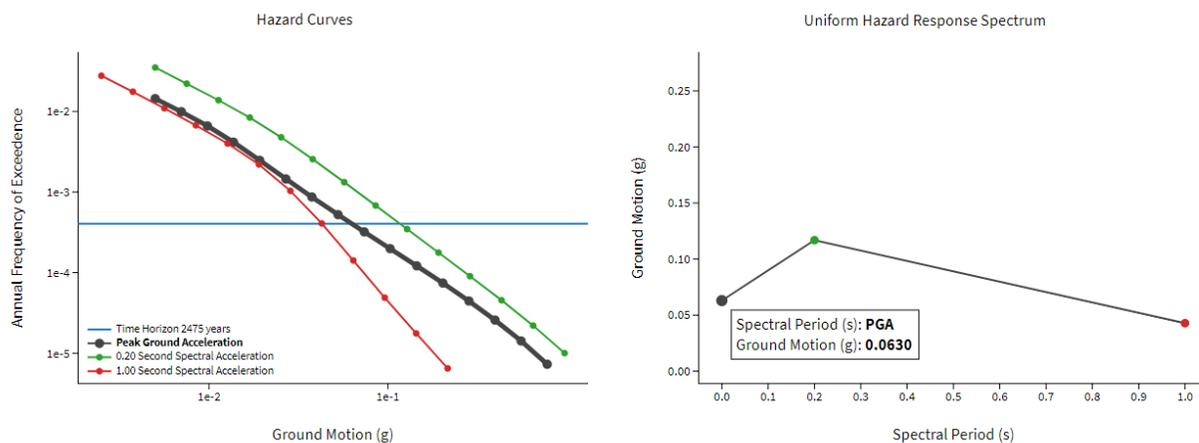
**Figure 1. Site-Specific Uniform Hazard Spectrum From USGS.**
