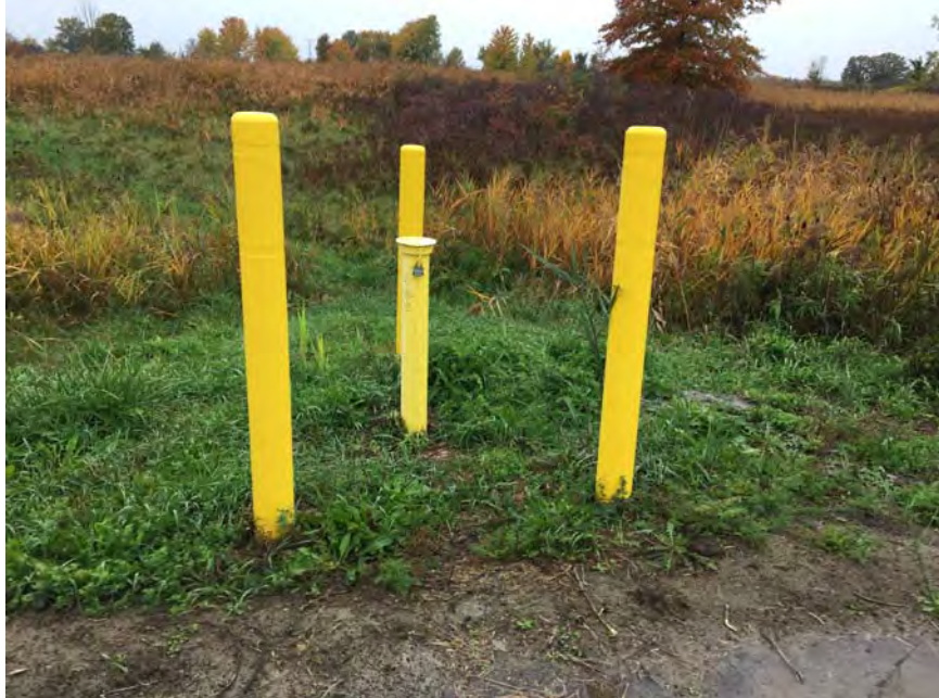
53. New CCR MW 16-01 Located Along Haul Road Inside Landfill Near Unconstructed Areas G3 and E.
