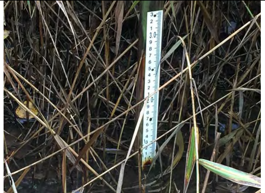
42. Perimeter Ditch Staff Gauge SG-12 Water Level Reading About 0.88 ft.
