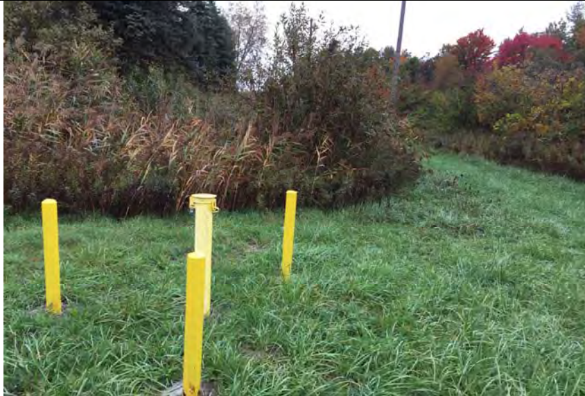
55. New CCR MW 16-03 Located NE Side of Landfill Outside of Slurry Wall and Perimeter Ditch
