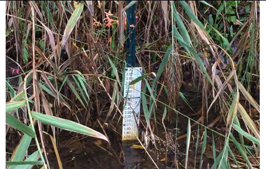
44. Perimeter Ditch Staff Gauge SG-01. Water Level Reading About 1.65 ft.
