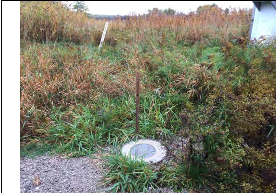
57. New CCR MW 16-05 Located on South Side of Landfill Outside of Slurry Wall at Construction Entrance Near Puttygut Road. Slurry Wall Marker Shown.
