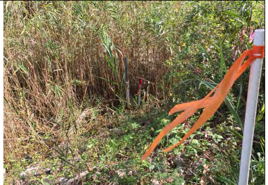
66. View of Perimeter Ditch Staff Gauge SG-10. Vegetation Heavy, but Review of Recorded Elevations Show Ditch is Still Flowing as Designed.
