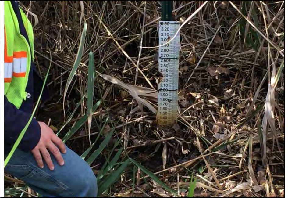
54. Perimeter Ditch Monitoring Staff Gauge SG-02. Gauge Numbering Not Visible. No Visible Flow.
