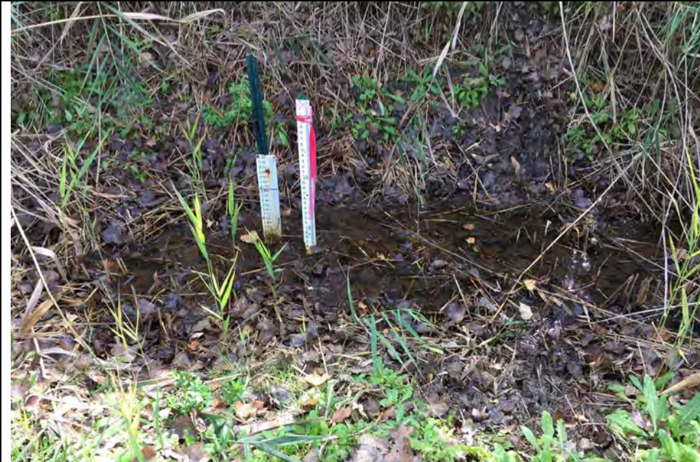
57. Perimeter Ditch Monitoring Staff Gauge SG-01. No Visible Flow Noted.
