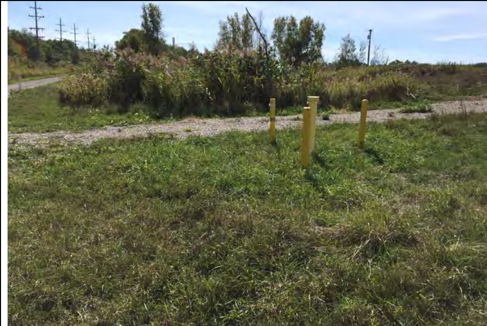
49. Typical View of One of Six Stick-up Monitoring Wells Around Perimeter of Landfill. Well is MW-16-02. One More Well is a Flush Type (MW-16-05).
