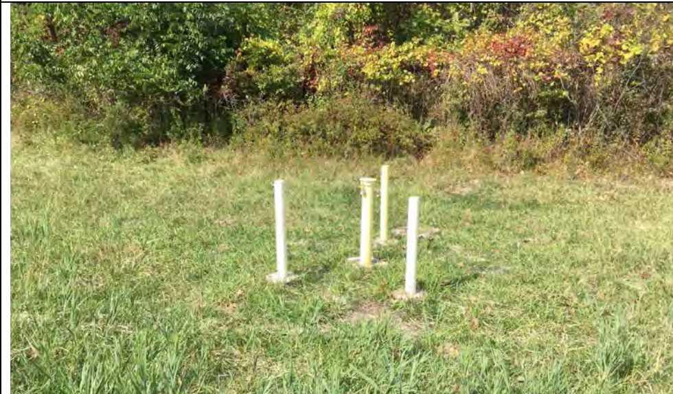
59. View of Monitoring Well MW-16-06. Access Clear and Well Protected.
