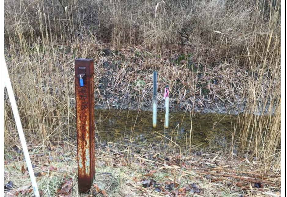
22. Looking at Perimeter Ditch Staff Gauge SG-02 and Piezometer PZ-1R. No Visible Flow in Ditch.
