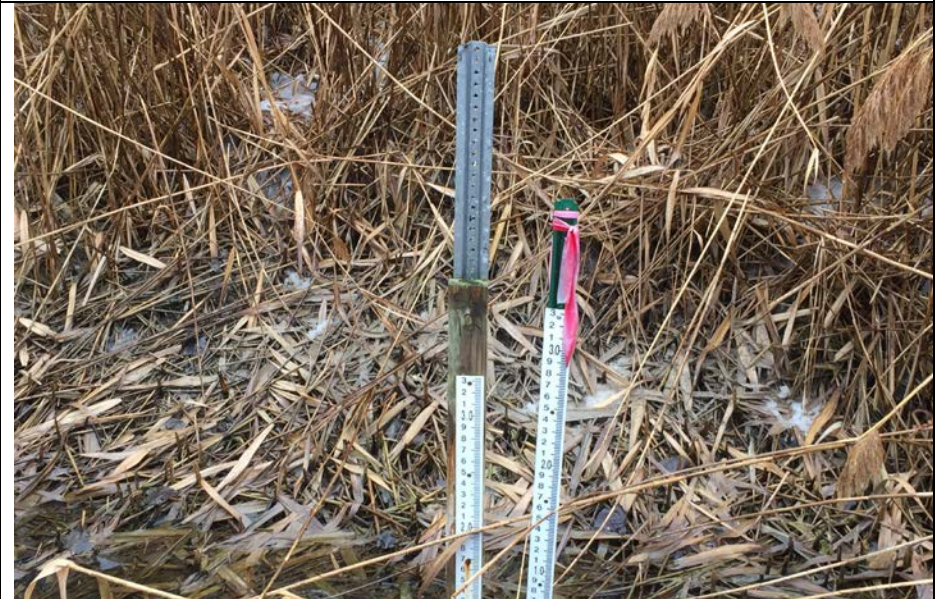
24. Close-up of Staff Gauge SG-12 and Perimeter Ditch with Heavy Vegetation. WL at Bottom of Photo. No Visible Flow.
