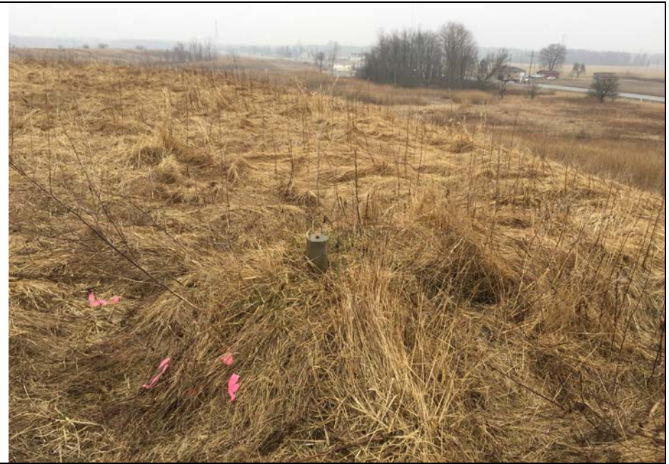
106. View of Construction Survey Monument Top of Closed Area F1 Along the West Slope.
