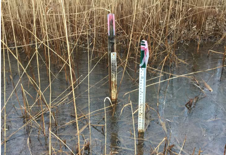
9. Looking at Perimeter Ditch Staff Gauge SG-07. Flow Observed Within Ditch.
