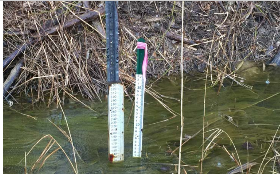
19. Looking at SG-03. Some Ditch Flow Observed.
