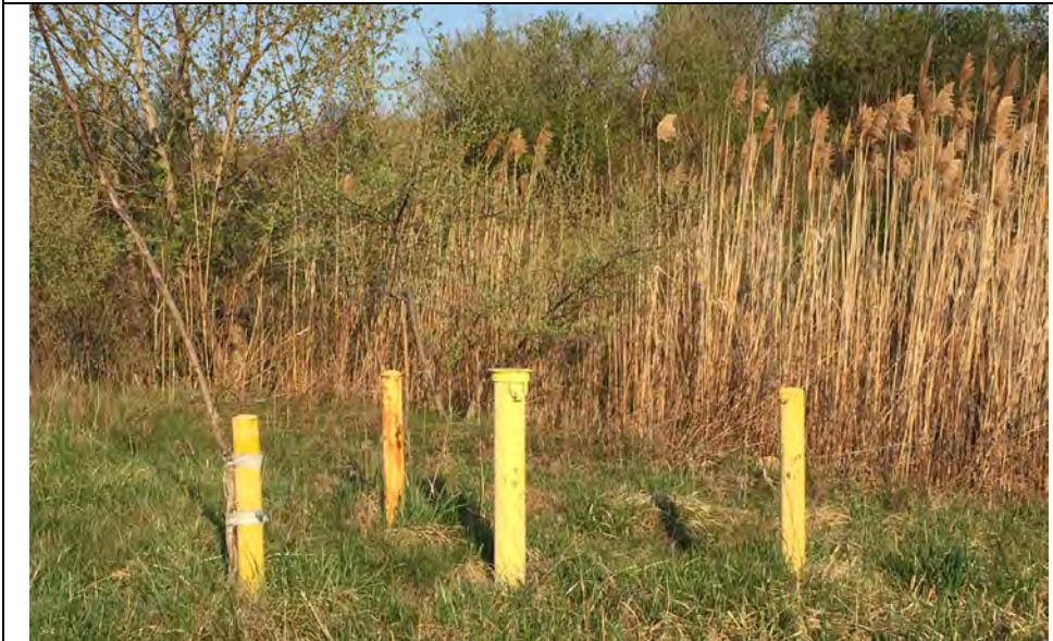
7. Monitoring Well 16-03. Well Protected and Cap Locked. Well Protection and Capping Typical of Inspected Above Ground Monitoring Wells.
