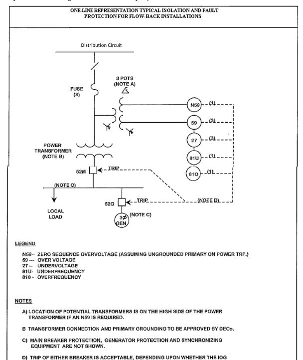
WANTS TO SERVE ITS OWN ISOLATED LOAD AFTER LOSS OF DECO SERVICE. IF GENERATOR IS SYNCHRONOUS, THE FIELD SHOULD ALSO BE TRIPPED.
